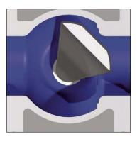
Plug is out of flow path when fully open
