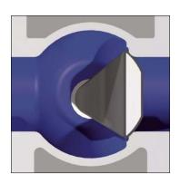
Plug rotates away from the seat for instant opening Seat wear and operating torque reduced No further seat contact until valve is closed again
