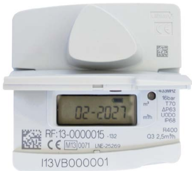
Static Water Meter LCD display
