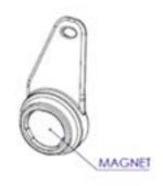
The MUT 7000 meter is equipped with a magnet for magnetic reed operation.
