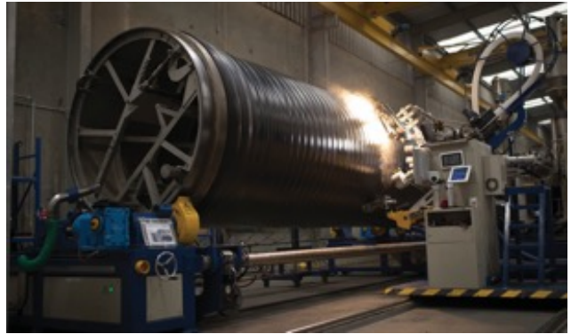
FIG. 1 Supaduct Rural manufacturing process.
