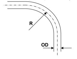
Table 3. Minimum field bend radius (pipe without ovality at 20°C)
