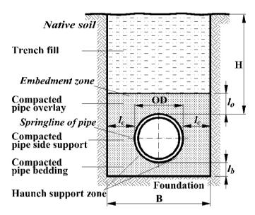
Fig. 1: Typical installation in a trench
