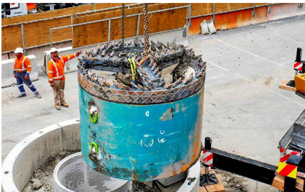
FIG. 4 Drilling head for TBM
