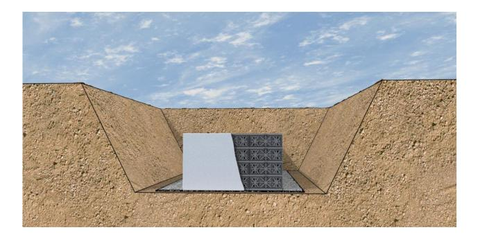
The excavation must also be designed in accordance with "Excavation pits and trenches" or similar standards. In particular, this includes the slope angle that has to be selected depending on the soil type for depths of  $\geq$  1.25 m.
