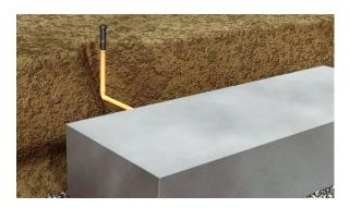
The required number as well as the size of the vents depend on the diameter of the inlet pipe and the number of inlets.
