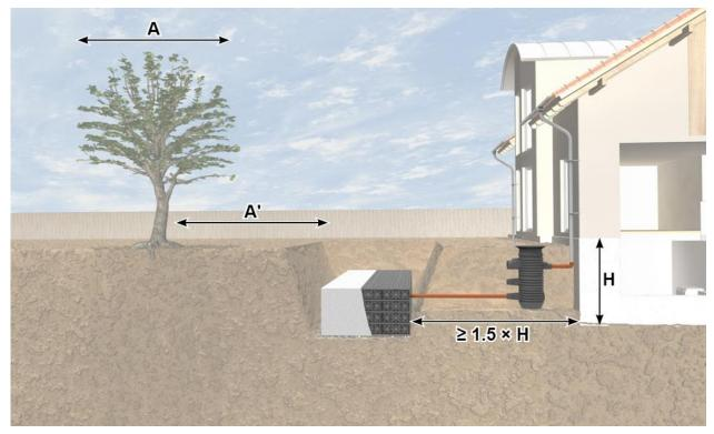
The distance between the installation base of an infiltration system and the average highest groundwater level expected must not fall below one metre according to most national standards. If this distance does fall below one metre, approval must be obtained from the relevant authorities.
