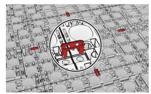
In the second and following layers, the modules are placed on top of modules already in place as shown.
