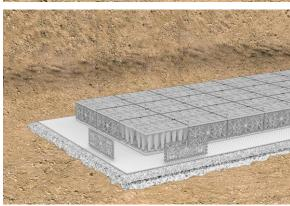
Once all the blocks are positioned, the system is fully wrapped in **geotextile**. This prevents the ingress of dirt particles into the system.
